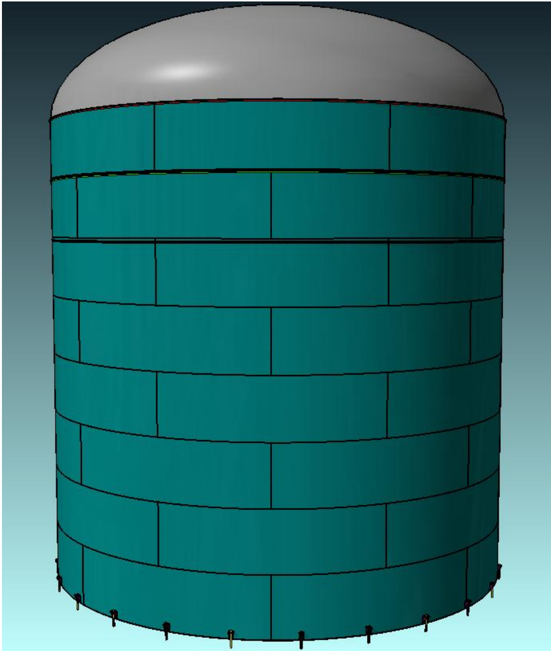
Figure 3.- Detail of the 3d design of a tank with dome roof, cylinder shell plates, top angle, 2 wind rings, bottom, annular bottom, anchor bolts and anchor chairs
