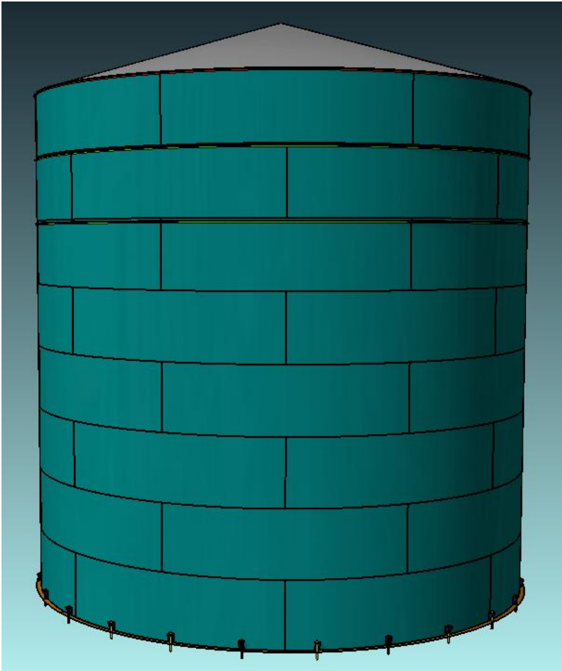
Figure 2.- Detail of the 3d design of a tank with self-supporting conical roof, shell plates in cylinder, top angle, 2 wind rings, bottom, annular bottom, anchor bolts and anchor chairs
